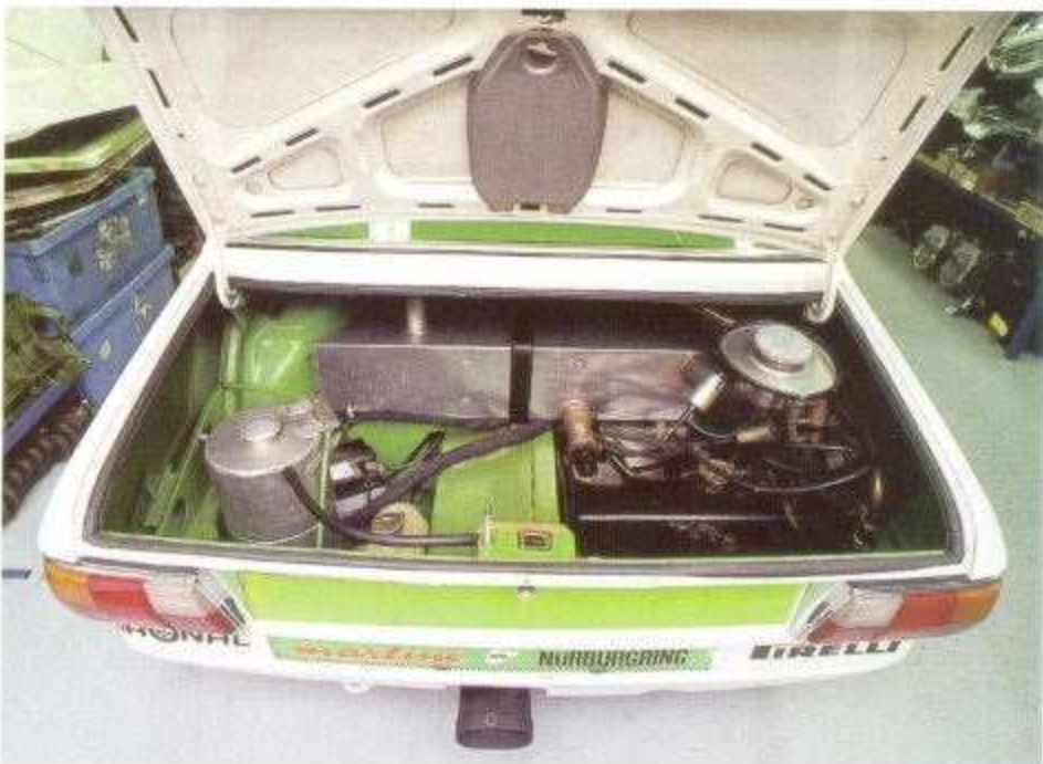
Above. Full-on race spec explains the 100-litre fuel tank and the oil tank on the left for the dry-sumped engine.
