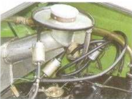
Above. Filler for boot-mounted fuel tank. Note the triple fuel pump arrangement.
