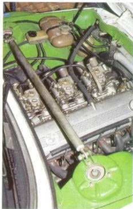
Above. Car was built in 1980 by Martini Racing. Right. Triple-Webered six makes around 340 bhp.
