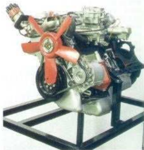
Above. Cutaway engine is a display unit from a dealer showroom. Before it went under the knife it was a 3-litre M30 unit from a 3.0CS.
