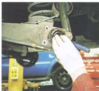
Semi-trailing arm loses its bearings...
