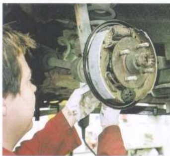
Handbrake cable back on and new shoes
