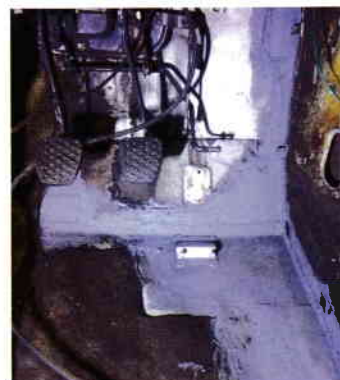
Repaired floor, with new throttle bracket
