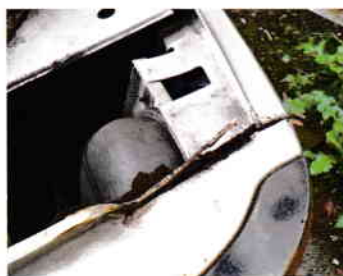
Corroded front wing seam had turned ugly
