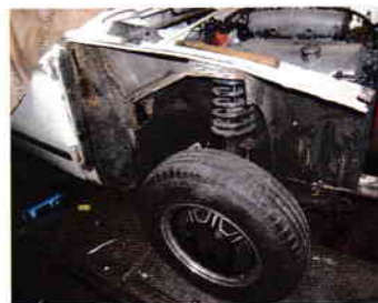
Hole in bulkhead had let water into cabin
