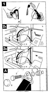
The 3-point safetyoelt with slide action buckle and dual sensitive emergency locking retractor is supplied with the fitting kit components
